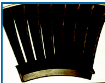
A) After 2360 operational hours, the blades behind 'brand X' are fouled -- and causing turbine output loss!
