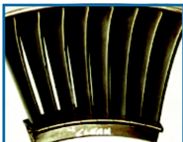
B) After 2360 operational hours, the blades behind the filters with Donaldson Spider-Web® are still clean -- and maintaining turbine output at optimal levels!
